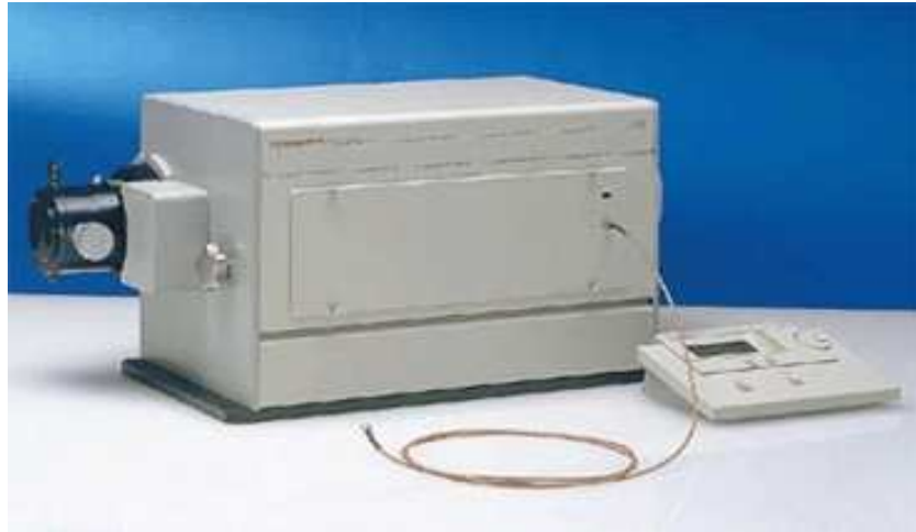
Figure 6: A Hamamatsu streak camera model C6860 with time resolution 500fs.
