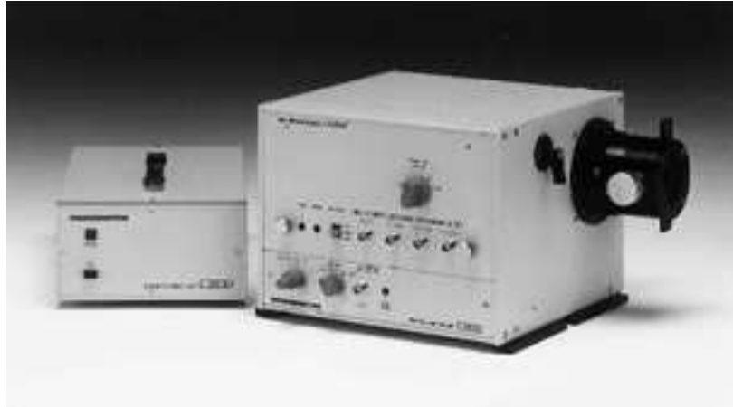
Figure 5: A Hamamatsu streak camera model C2830 is shown here which is very similar to the C1587 that it was actually used.
