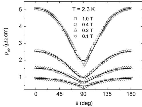
**FIGURE 1.** Resistivity  $\rho_{ab}$  vs angle  $\theta$  measured at 2.3 K. The solid lines are fits of the data with Eq. (3).
