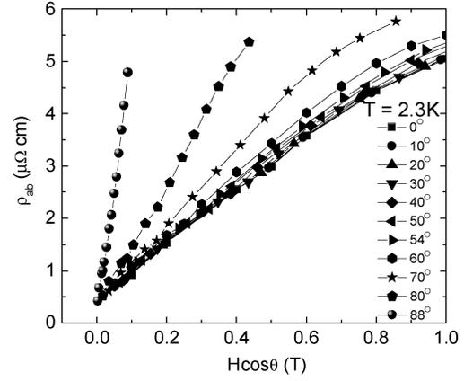
FIGURE 2. Resistivity  $\rho_{ab}$  vs the perpendicular field component  $H\cos\theta$ , measured at 2.3 K and fixed angles  $\theta$ .
