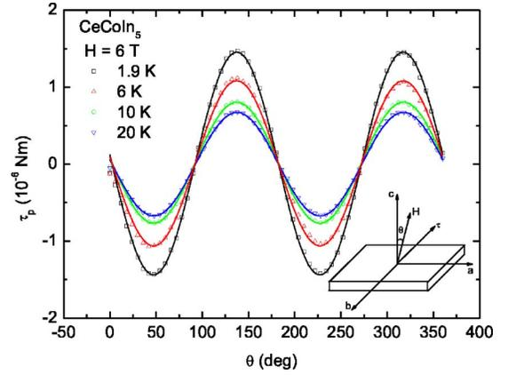
FIG. 1. (Color online) Angular  $\theta$  dependence of the paramagnetic torque  $\tau_p$  measured in the normal state of CeCoIn<sub>5</sub> at different temperatures  $T$  and applied magnetic field  $H$  values. The solid lines are fits of the data with Eq. (1). Inset, sketch of the single crystal with the orientation of the magnetic field  $H$  and torque  $\tau$  with respect to the crystallographic axes.
