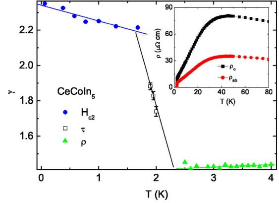
FIG. 7. (Color online) Composite plot of the temperature  $T$  dependence of the anisotropy  $\gamma$ . The circles show the results obtained from the upper critical field data (Ref. 26), the triangles are obtained from the resistivity data shown in the inset of this figure, and the squares are from the present torque data measured in an applied magnetic field of 0.3 T. Inset,  $T$  dependence of the in-plane  $\rho_a$  and out-of-plane  $\rho_c$  resistivities measured in zero field.
