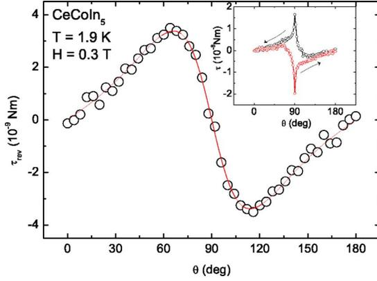
FIG. 4. (Color online) Angular  $\theta$  dependence of the reversible torque  $\tau_{\text{rev}}$ , measured in the mixed state of CeCoIn<sub>5</sub> at a temperature  $T$  of 1.9 K and an applied magnetic field  $H$  of 0.3 T. The solid line is a fit of the data with Eq. (9). Inset,  $\theta$  dependence of the hysteretic torque  $\tau$ , measured in increasing and decreasing angle at the same  $T$  and  $H$ .
