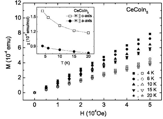
FIG. 3. Plot of the magnetic moment  $M$  vs applied magnetic field  $H$ , with  $H \parallel c$ -axis (solid symbols) and  $H \parallel a$ -axis (open symbols), measured at 4, 6, 10, 15, and 20 K. Inset, susceptibility  $\chi$  vs temperature  $T$ , measured with  $H \parallel c$ -axis and  $H \parallel a$ -axis.
