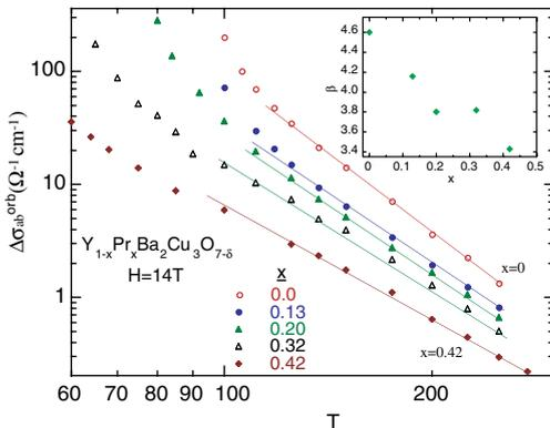
Fig. 1. Log–log plot of orbital magnetoconductivity  $\Delta\sigma_{ab}^{orb}$  vs temperature  $T$ . Inset: exponent  $\beta$  vs Pr content  $x$ .
