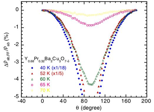
Fig. 2. Plot of flux-flow-like magnetoresistivity  $\Delta\rho_{ab,FF}/\rho_{ab}$  vs angle  $\theta$  of  $Y_{0.68}Pr_{0.32}Ba_2Cu_3O_{7-\delta}$  measured at 60, 65, and 70 K. For comparison,  $(\Delta\rho_{ab,FF}/\rho_{ab})(\theta)$  in the superconducting state (40 and 52 K) are also shown with filled symbols.
